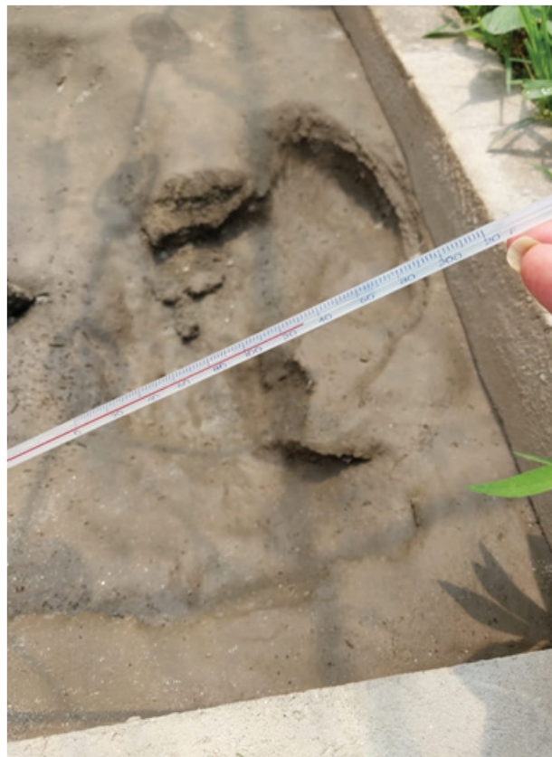
Figure 4.2: Temperature measured to be 130.5^{\circ}\text{Fahrenheit} = 54.72^{\circ}\text{C}
